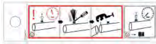
940 - "Transportation filling" warning sign next to Schrader valve
